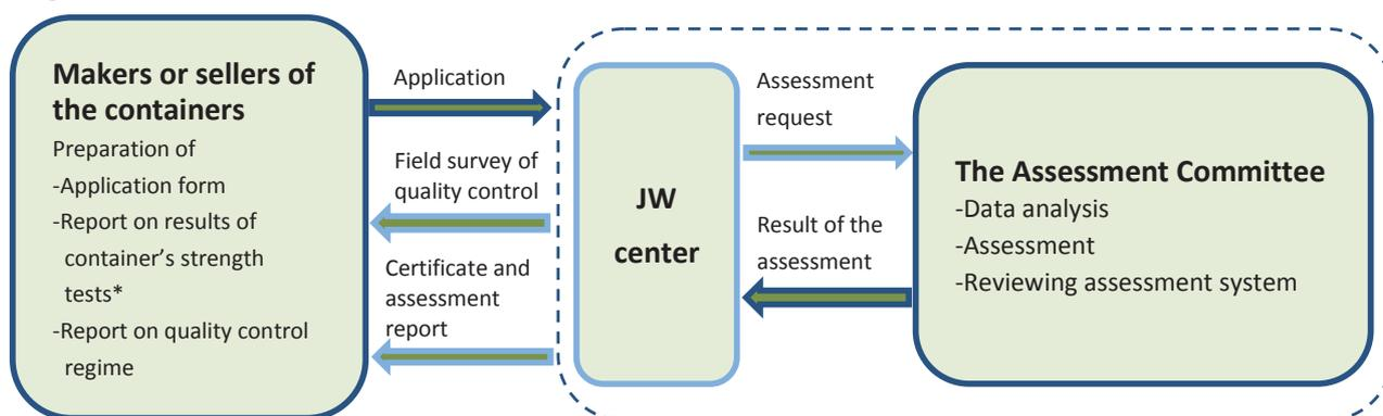
\*Container's strength tests: Penetration resistance test, Dropping test, Stacking test, Toppling test, etc.
